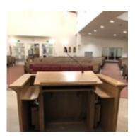
9. Even the ambo is created for accessibility, with a simple hydraulic lift that lowers the height for wheelchair accessibility. The rails allow for rolling straight up and are strong for a person to use for pulling themself to standing position.
